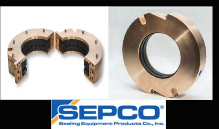
The SEPCO Air Seal-(SAS), is an engineered pneumatic sealing system designed to seal the shafts of equipment where typical contact seals, such as packing or mechanical seals are ineffective and often too costly to operate and maintain. A true "non-contact" air seal designed for wet or dry applications, the seal is particularly successful in difficult-to-seal applications such as powder and bulk solid processes.
